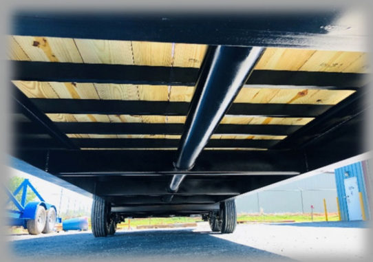
12" I-BEAM FRAME W/ 4" ANTI-TWIST PIPE, 16" ON CENTER CROSS-MEMBERS
