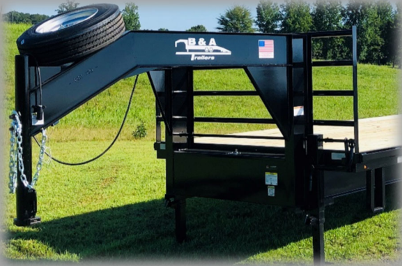
SPARE TIRE, DUAL JACKS, LOCKING TOOL BOX, BOARDING STEP, PIPE BULKHEAD
