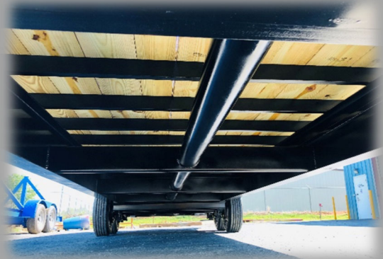
12" I-BEAM FRAME W/ 4" ANTI-TWIST PIPE, 16" ON CENTER CROSS-MEMBERS
