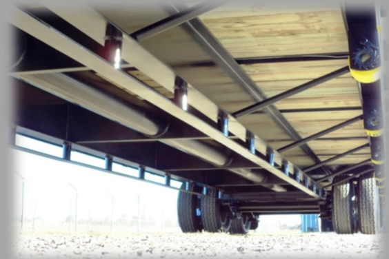
12" I-BEAM FRAME, TRUSS & ANTI-TWIST PIPE, PIPE TO SIDE BRACES
