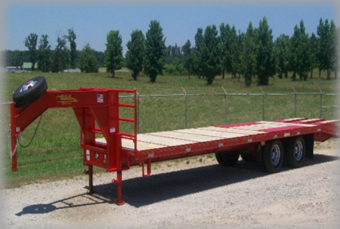
12" I-BEAM FRAME – 102" WIDE 34" DECK HEIGHT
