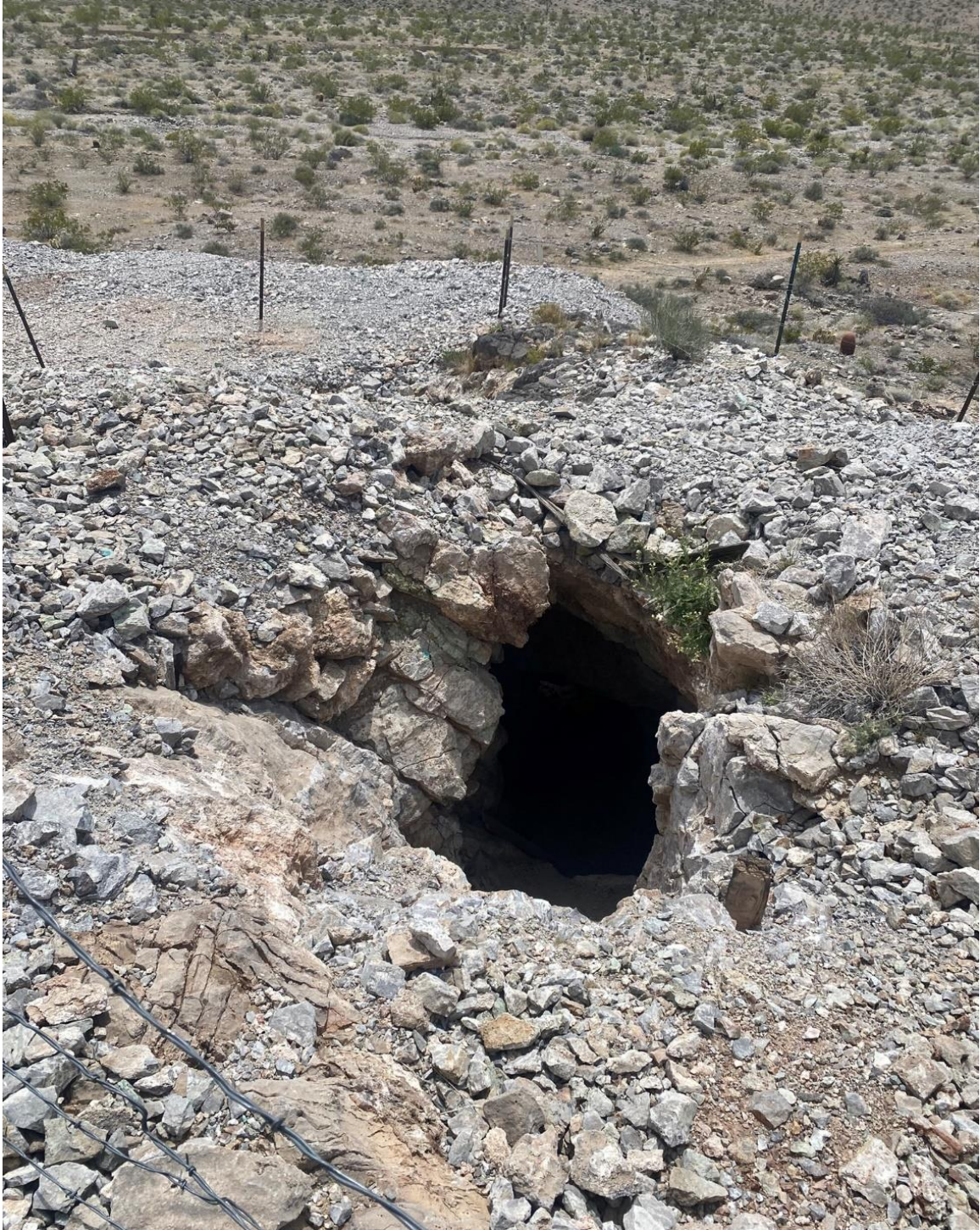
Photo 6: Photo, top of inclined raise at the Desert valley prospect. A high-grade Cu, Ni and Co chip sample was collected from in place vein mineralization of the left-hand side of this raise or stope.
