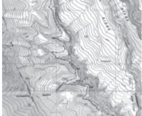
e. Valley – A valley is level ground bordered on the sides by higher ground. Contour lines indicating a valley are somewhat U-shaped.
