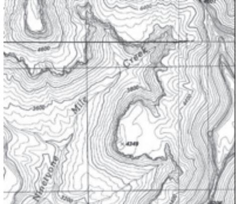
d. Cliff – A cliff is a near vertical slope. The closer the lines are to each other, the steeper the slope. A cliff will be shown on a map by the close contour lines that touch or have tick marks on them. These tick marks will point towards the lower ground
