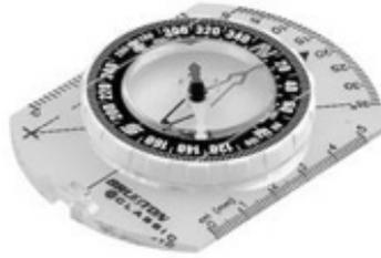
3. Calculating the Back Azimuth. To calculate what the bearing is from that object back to you is a simple matter of subtracting 180 degrees from the original azimuth if it is more than 180 degrees, or adding 180 degrees to the original azimuth if it is less than 180 degrees.
