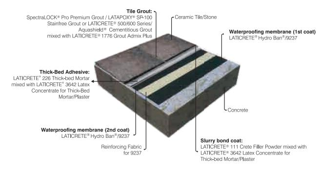
Note: LATICRETE® Hydro Ban® does not require use of Reinforcing Fabric
