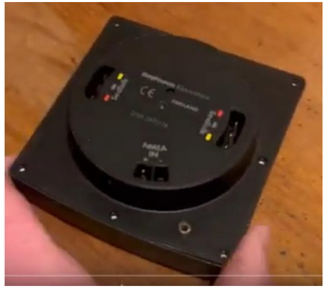
Figure 10 Remove the 8 small screws on the back and pry by hand apart.
