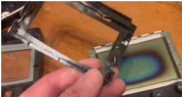
Figure 12 Remove the frame that holds the LCD screen in place
