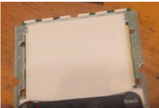
Figure 13 Unplug the LCD display by pulling it straight up
