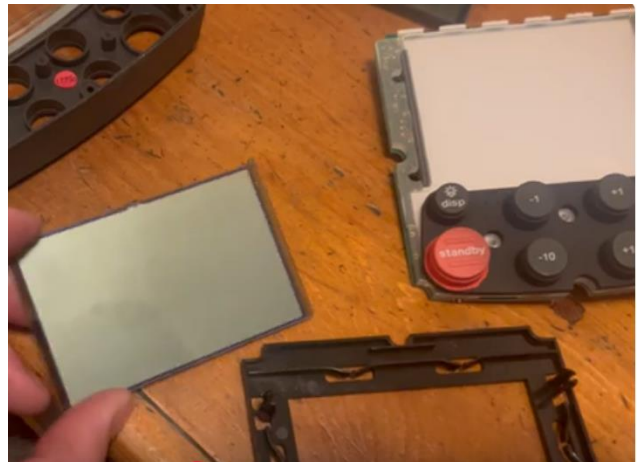
Figure 14 Place the new screen in the frame and then press it onto the circuit board and reassemble.
