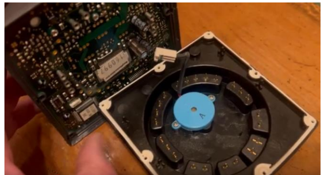
Figure 11 Pry the back circuit board off and disconnect the connector, and then the 3 screws that hold the circuit board to the display.
