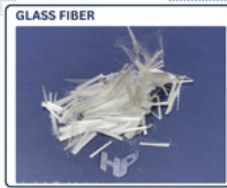
12mm Glass Fiber Strands Add 100 Grams in 1 Bag Cement
