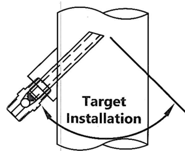
Vertical Pipe Installation
