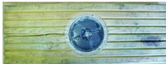
Figure 1 - Damage of SolarEye 80 product in decking following a compressive load of 600kN
