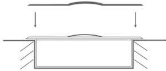
We re-engineered the standard product by adding a little hat to reduce the upwards light spillage by around 98% whilst remaining the same in profile, making the 'Bat Hat' a far friendlier option.
