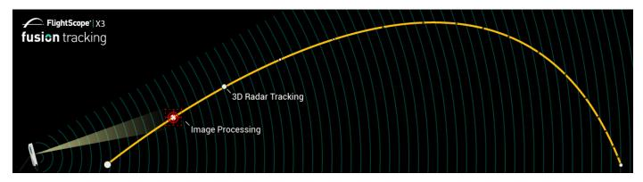
Fusion Tracking = Tracking Radar + Image ProcessingFusion Tracking is an innovative combination of 3D Doppler tracking and image processing. Technological advances in the field of image processing made it possible to improve the already accurate 3D tracking radar data for both club and ball measurements.
