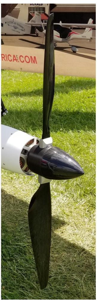
The prop automatically adjust to Amps, air speed and rpm for take off, feather and airbrakes.
