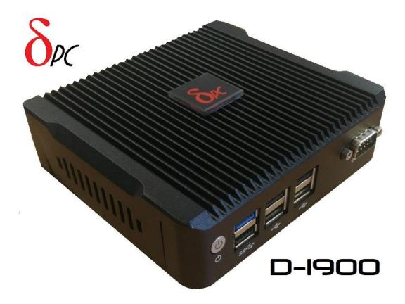
The Delta D-1900 provides exceptional reliability for the most challenging environments. Well tested in hot, dusty conditions on more than one continent, the D-1900 delivers where other normal PCs fail. Utilising a fan-less chassis with no moving parts to ensure reliability, the Delta D-1900 make this a maintenance free computer and a sensible choice for your most challenging projects. (Perfect for UK schools due to the much lower cost of power consumption!)
