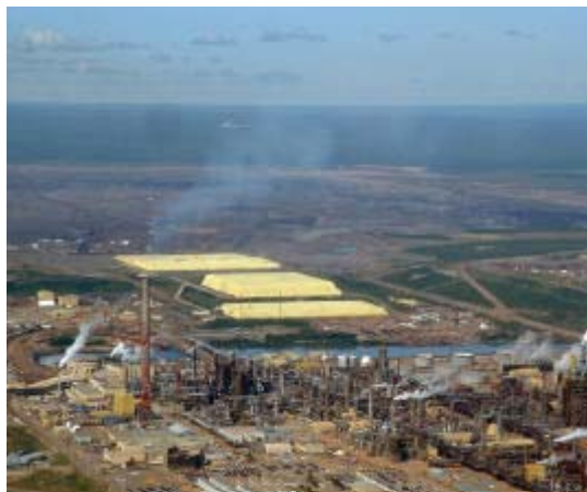
One of the environmental benefits of a bio-heapleach metals mine is that it consumes massive amounts of sulphur during normal operations. The bright yellow sulphur pyramids stockpiled in this aerial photo near Fort McMurray, Alberta, are part of the waste byproducts created when heavy oil is upgraded. Photo courtesy: DNI Metals Inc.
