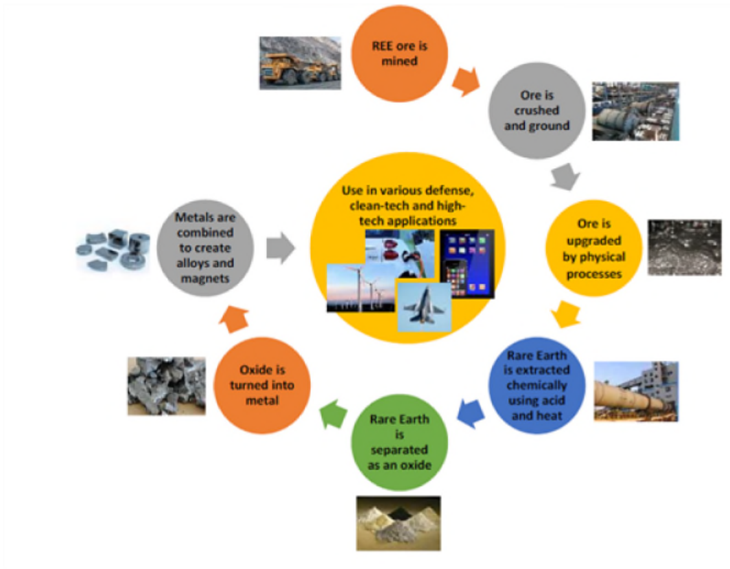
Figure 2: Schematic diagram of the metallurgical processing required to produce REE products from ore
