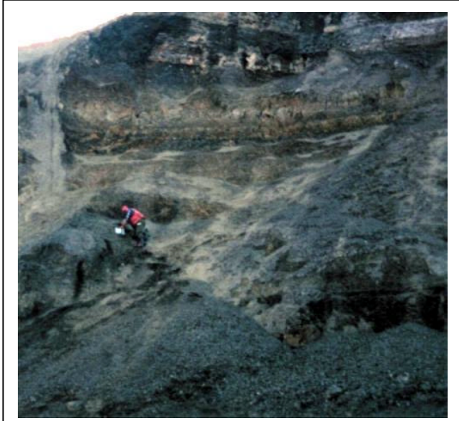
Plate 2: Typical stratigraphic section and related slump, Cretaceous Shales, Birch Mountains, Alberta. (Repel mapping by the author)
