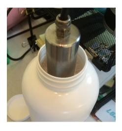
b) Using the **P78** sensor, samples were poured into the plastic sample cup that was attached directly in front of the sensor head. Because the sensor averages 40 readings a second, any packing or flow variations can be mitigated by signal smoothing using the Liebherr controller or an end users PLC.
