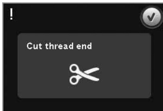
9. When the first color is completed, your machine stops. A pop-up appears asking you to change color. Re-thread with the next color and continue embroidering by pressing start/stop. Each color segment is tied off at the end and the needle thread is cut.
