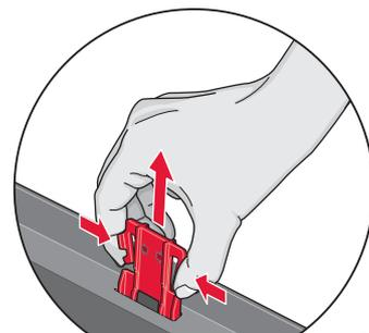
*When removing the embroidery unit from the box for the first time, be sure the shipping brace on the underside of the embroidery unit has been removed.*
