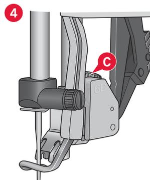
To remove the embroidery foot loosen the screw (C), squeeze the embroidery foot together and pull it out to the right. Tighten the screw.
