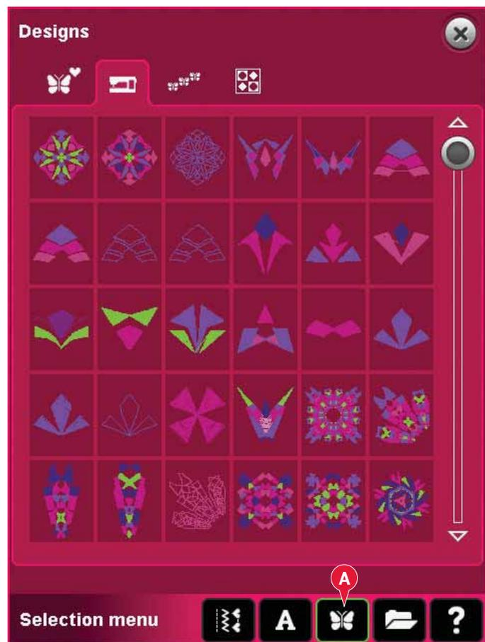
3. The machine automatically switches to Embroidery edit. The design is placed in the center of the hoop.
