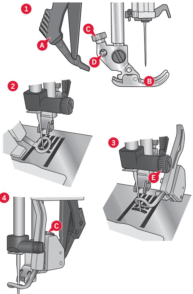
To remove the embroidery foot loosen the screw (C), squeeze the embroidery foot together and pull it out to the right. Tighten the screw.
