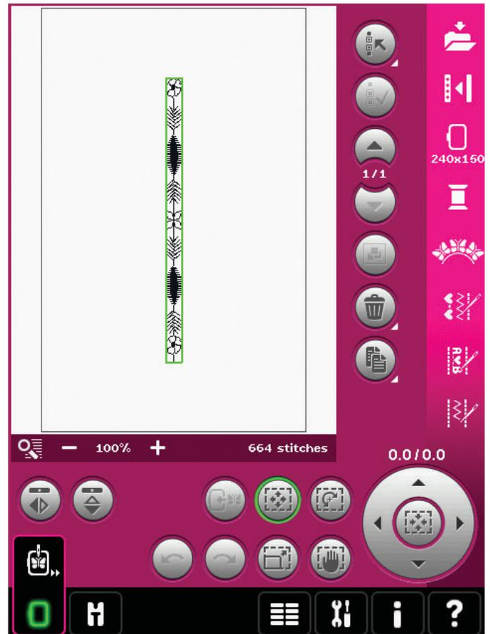
4. Deselect the sequence by touching outside the design on the screen, or step by using the arrows.
