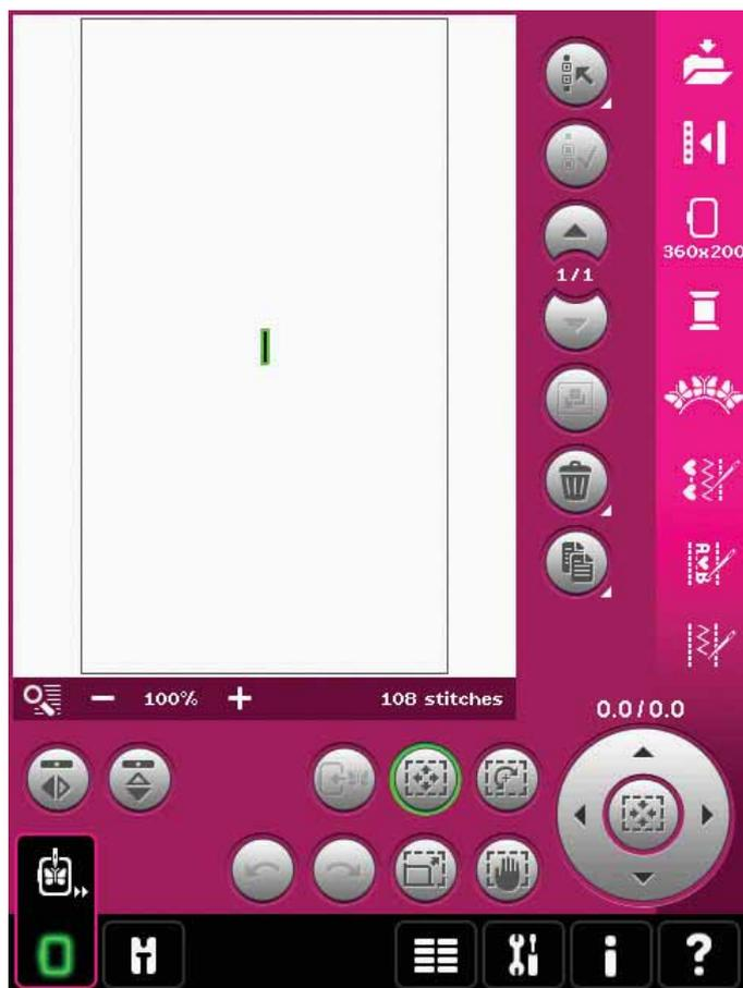
2. Open Basic Shape Creator™ feature. Select the straight line from the list (A). Select touch function - rotate, and then touch the wheel center one time to rotate the baseline 90 degrees.
