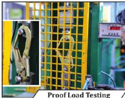
Proof Load Testing
