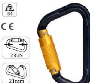
Ref. PN 117 F Aluminium Quarter Turn-locking Karabiner (Forged)
