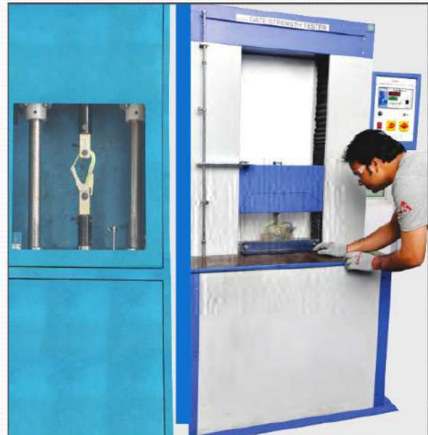
Static Strength testing on randomly drawn samples, lot wise for major axis, minor axis, gate side, strength and gate-face strength as per requirement.
