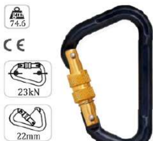
Ref. PN 116 F Aluminium Screw-locking Karabiner (Forged)
