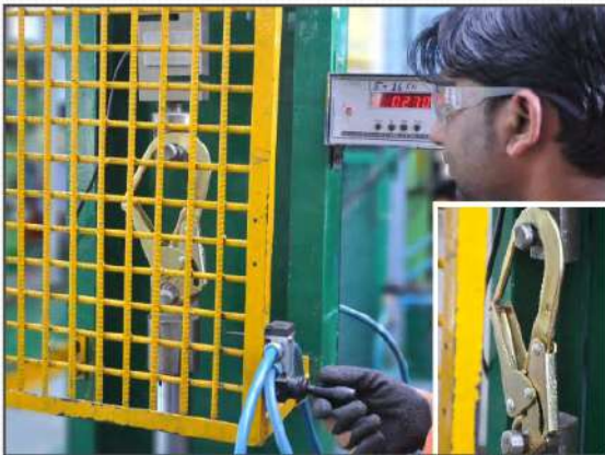
100 % proof load testing at 16 kN post assembly of components.
