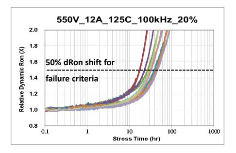
Reference: "New Circuit Topology for System-Level Reliability of GaN" (ISPSD2019)
