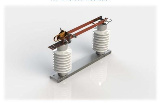
The HPL switch is a two-insulator vertical break single phase hook stick design. Single phase operation is accomplished with the use of a hot-stick. Operation of the switch is accomplished through a pry-out paddle from the high pressure line (HPL) contact arrangement. Copper components are utilized throughout the design. The HPL is also available in a "V" configuration.
