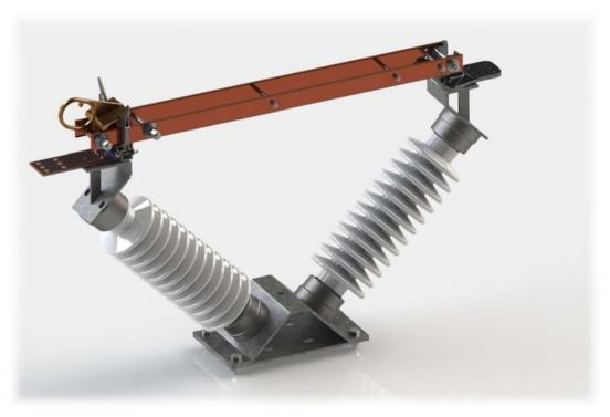
The HPL-V switch is a two-insulator "V" slant break single phase hook stick design. Single phase operation is accomplished with the use of a hot-stick. Operation of the switch is accomplished through a pry-out paddle from the high-pressure line (HPL) contact arrangement. Copper components are utilized throughout the design.
