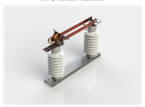
The HPL switch is a two-insulator vertical break single phase hook stick design. Single phase operation is accomplished with the use of a hot-stick. Operation of the switch is accomplished through a pry-out paddle from the high pressure line (HPL) contact arrangement. Copper components are utilized throughout the design. The HPL is also available in a "V" configuration.
