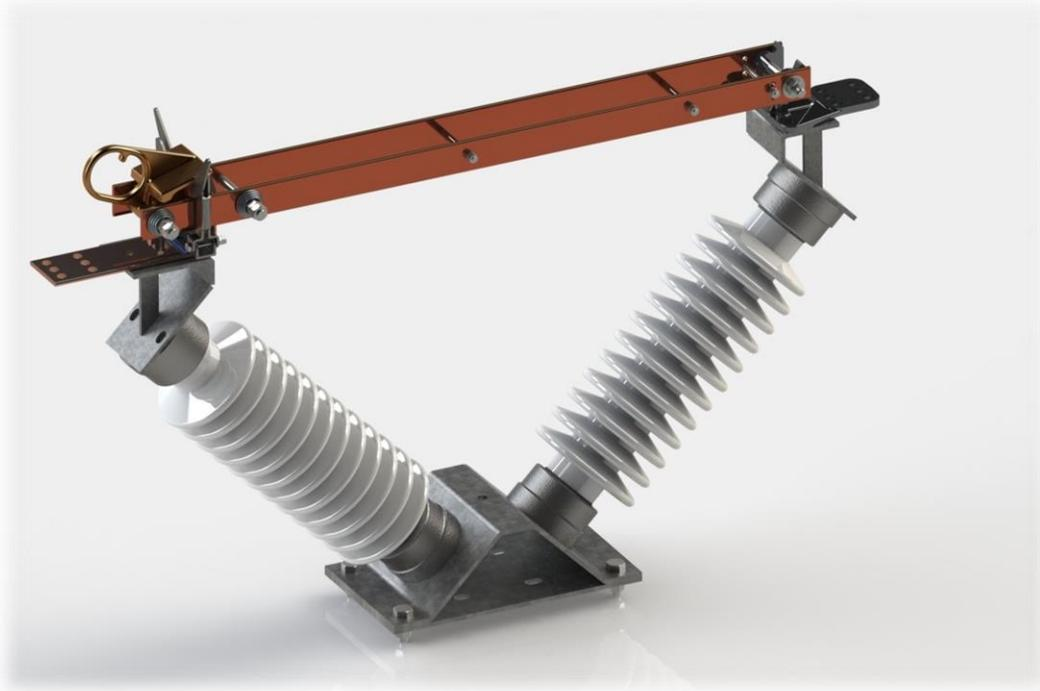
The HPV switch is a two-insulator “V” slant break single phase hook stick design. Single phase operation is accomplished with the use of a hot-stick. Operation of the switch is accomplished through a pry-out paddle from the high pressure line (HPV) contact arrangement. Copper components are utilized throughout the design. The HPV is also available in an “L” parallel configuration.
