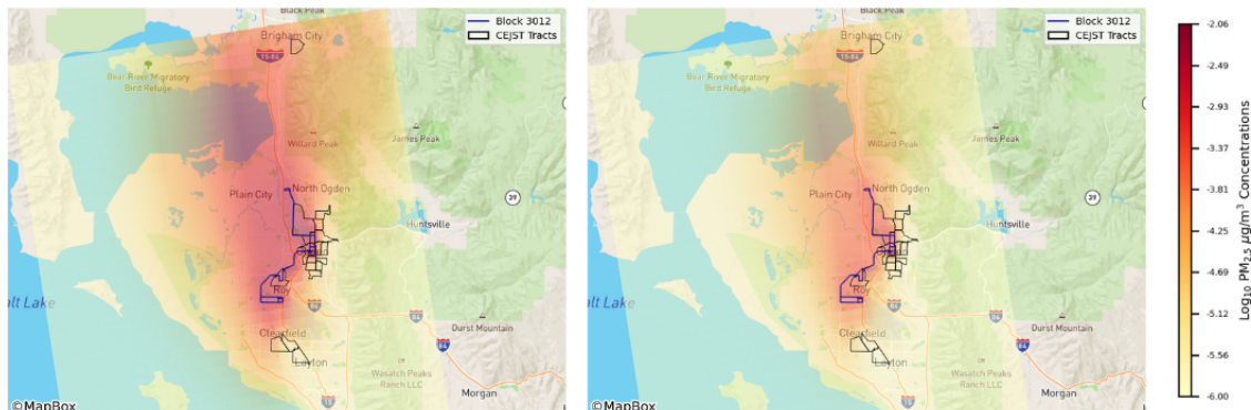
Figure 3.8. Block 3012 and its emissions plumes. Left: Diesel bus; Right: Electric bus.
