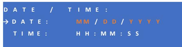
To change the DATE first you will see that DD (Days) flashes, modify the value with the arrows buttons and press the ENTER button, it will flash MM (Months), modify the value with the arrows buttons and press the ENTER button, it will flash YYYY (Years), modify the value and press the ENTER button, the new values will be recorded. If you press the ESC button at any point in the process, the changes will not be recorded.
