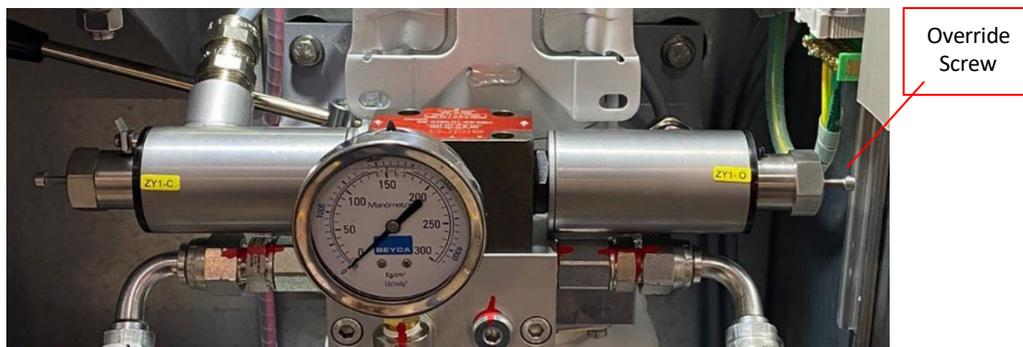
3° Once the previous step is completed, operate the manual pump using the indicated lever. It is important to monitor the pressure using the gauge while performing manual pumping and ensure it does not exceed 2000 psi (maximum actuator pressure).
