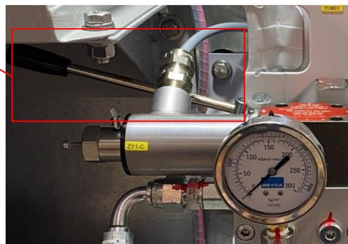
4° Once the manual pumping process is complete, the override screws should be loosened and ensured that they are not sufficiently engaged to lock the system in NORMAL mode.
