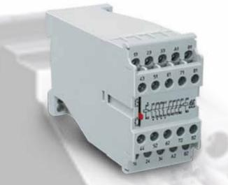
Latching/interface and switching relays are ideal connecting links between the highly-sensitive and low-power logic circuitry of a PLC, control system or process computer and the raw environment of the power level on a machine such as motor drives, magnetic clutches or hydraulic cylinders. The relays ensure a metallic isolation between logic and power circuitry.
