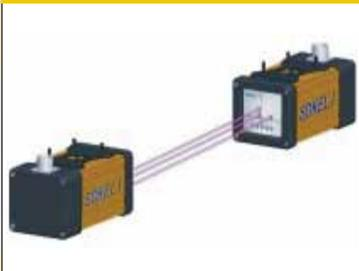
Ideal for Press Brake point of operation guarding, tested and certified TYPE 4 with TUV. Independent OSSD outputs, Detection range up to 20 meters, ideal protection for bending small and complicated parts and optional control box for folding box and muting mode.
