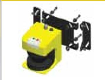
Two dimensional optical detection device for personnel and machine safety. Protection zone of 4 meters with an angle of 190 degrees. Minimum object sensitivity is 7cm at 4 meters. Protective and warning zones can be configured into complex and irregular zones through programming.
