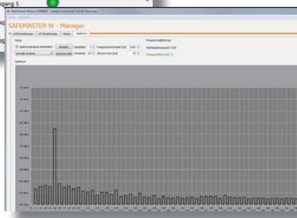
► **Spectrum analysis** (the integrated Spectrum Analyzer provides a quick overview of all available channels)
