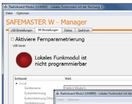
► **Display** (device labeling, set frequency range 433 MHz or 869 MHz, received transmission power)
