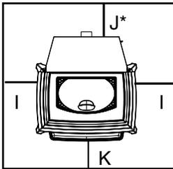
Use a noncombustible floor protector extending beneath appliance and to the front/sides/rear as indicated. Measure front distance (K) from surface of glass door. Approved for use with Type 1 hearth pad.
