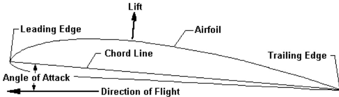
Lift increases as the velocity of the air passing over the wing increases or as the angle of attack increases as long as the flow of air over the wing remains smooth. Actual flight is attained when the force of the lift equals weight.
