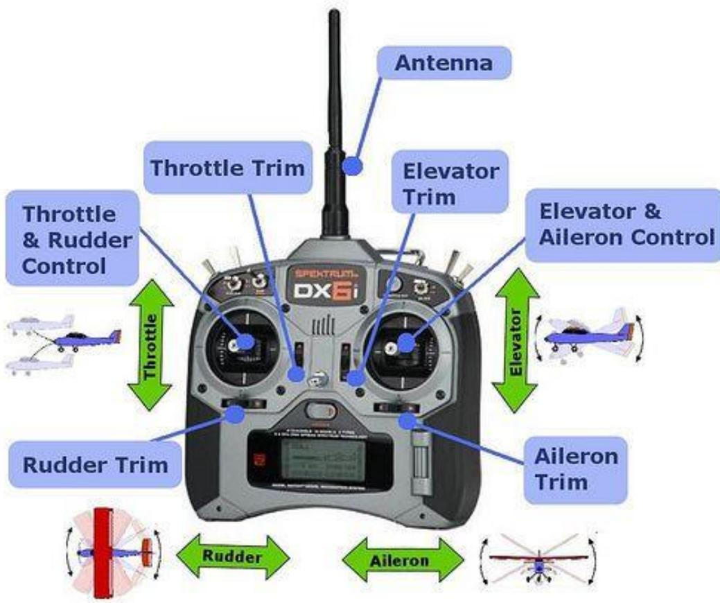
This is a typical lay-out of the transmitter and its functions.
