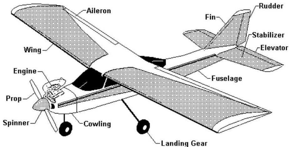
**Aileron** – The moveable portion of the wing which causes a change about the roll axis.
