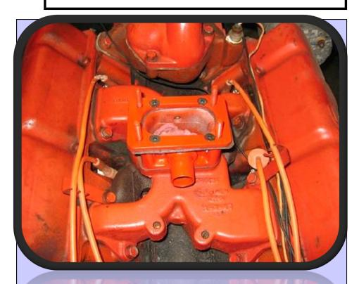
Above: A 305 V6 showing how the spark plugs are located next to the intake manifold for easier maintenance.
