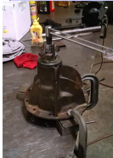
side adjusting screw until it just touches the ring gear. Now screw in the opposite side adjusting screw until snug against the bearing. At this point rotate the ring gear and pinion to check for tight spots. If too loose back off the adjusting nut opposite the ring gear and adjust the ring gear side adjusting nut to the point where it takes a bit of effort to rotate the assy.
