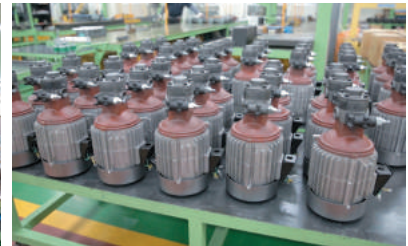
▲ T-rotor pump 조립 Line
