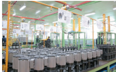
▲ Coolant pump 조립 Line
