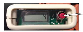
Press the RESET button, through the access hole to reset the counter.
