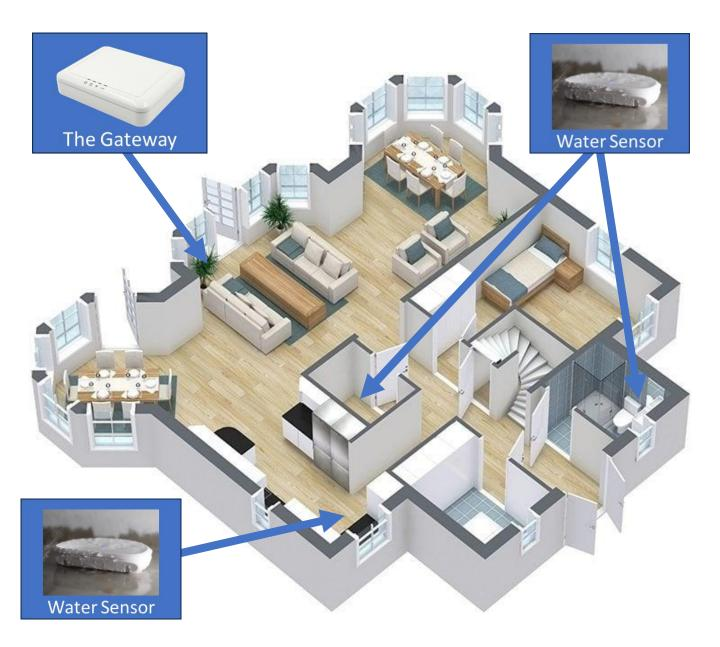
Water sensors report wirelessly to the gateway and then on to your cell phone. Water sensors will operate for several years on the same battery.
