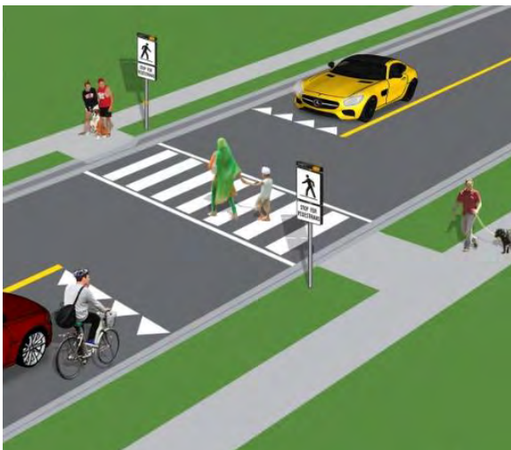
Figure 7.6: Diagram of PXO with Ladder Stripes, Signs and Pedestrian-Activated Lights.
