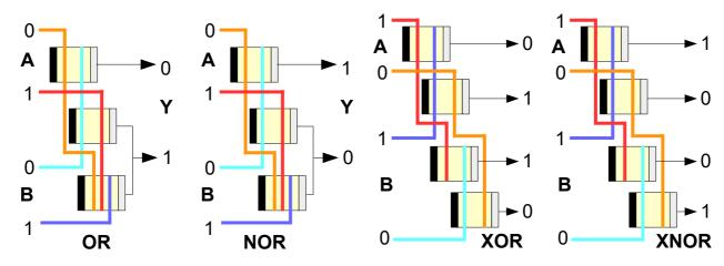
Another notable advantage of DSOLA circuits is that while most current laser applications require a strong output, the laser-threshold transistor operates with just enough energy to half activate the threshold of the next transistor. This significantly reduces the output power necessary lowering the energy consumption and heat generation, particularly at the nanoscale.
