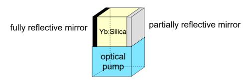
The laser-threshold transistor operates as an optical switch, emitting an output laser beam only when two input laser beams are present simultaneously. The gain medium is optically pumped just below the lasing threshold (a). Each input laser beam alone lacks sufficient power to initiate lasing (b, c), but when combined, their total power exceeds the threshold, activating the Yb:Silica laser (d) producing an output beam through the partially reflective mirror.
