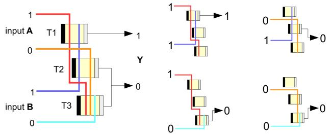
The NAND gate shares the same composition and function as the AND gate, with the key difference that T1 outputs to Y0, while T2 and T3 output to Y1.
