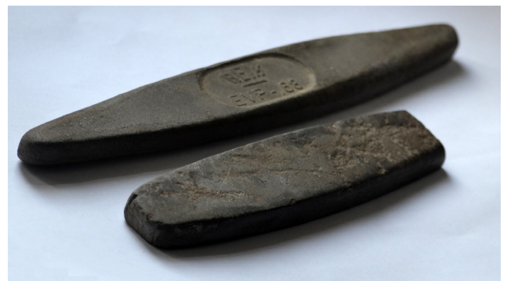
Figure 4. A traditional natural heavy used Whetstone (bottom) compared with an artificial whetstone (top).
