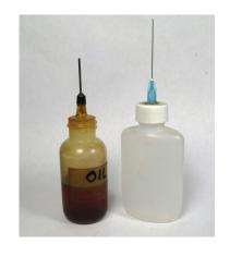
I use one with a short length of tubing for oil when I'm sawing or when drilling harder metals like steel. Another bottle I found in a plastics store has a longer length of metal tubing on it. Plastics people use them for dispensing fast drying glues to join pieces of
