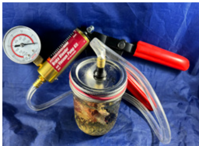
Homemade vacuum pot using a mason jar, valve stem and brake bleeding pump.
