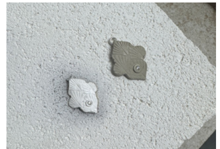
Metal clay pieces before firing, right, and after firing, left. Notice the reduction in size after firing.
