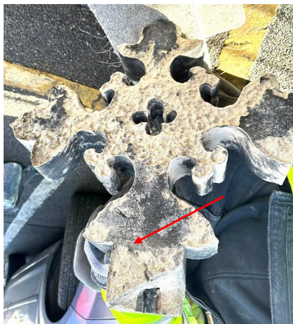
Photo 9 Cross after removal – note half of base (arrowed) fell away when cross lifted
