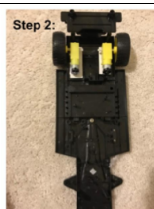
Motor and Wheels installed in the frame
