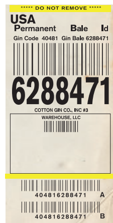
PBI tag: The first two digits of the gin code identify the classing office, followed by three digits identifying the gin. The remaining seven digits identify the bale.
