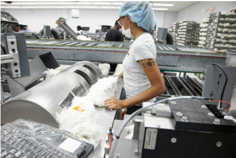
Fiber length and strength measurements are made on the same “beard” of cotton.
