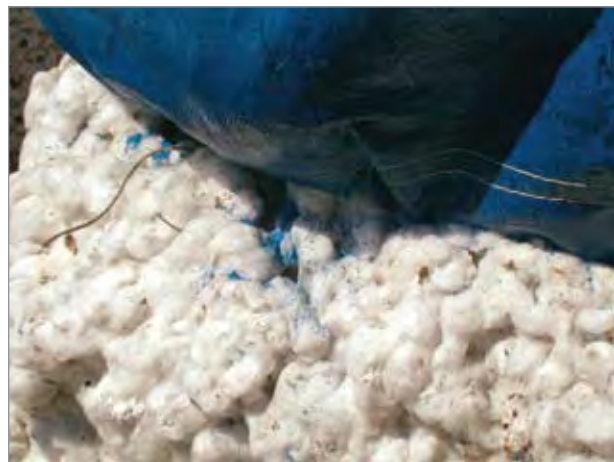
Figure 21. Coating breakdown due to extended UV exposure can cause contamination of cotton lint. The blue color on the cotton is flakes of coating that have been caught in the lint.
