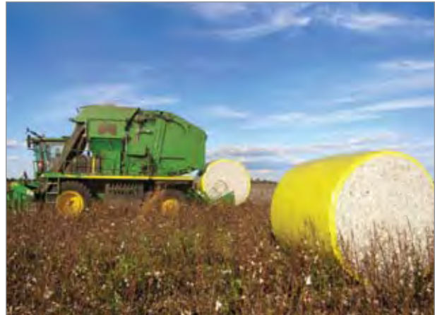
Figure 16 A John Deere 7760 cotton picker carrying a finished round module while harvest continues and the next module is being formed.
