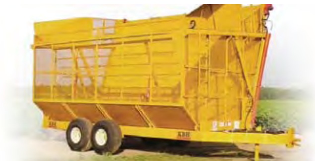
Figure 2 The boll buggy is used to transport harvested cotton between the harvester operating in the field and the module builder located at the edge of the field. (Photo courtesy of KBH, Inc.)
