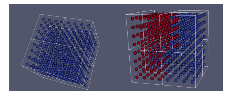
The diagram below shows the physical construct of an optimized 3D Torus (16x16x16), as well as a representative example of topology slices. A total of 64 cubes, with 64 nodes each, forms a 4k (4096) node cluster as a single availability zone (AZ) with three additional AZs possible, bringing the overall datacenter capacity to 16k nodes.
