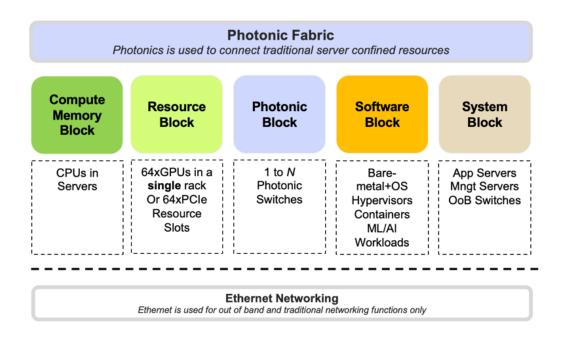
We use software to control and facilitate the how nodes (i.e. CPU + Resources) are constructed within the DX fabric.
